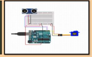
Aurdino Uno R3 :- The Arduino Uno R3 is a microcontroller board based on the ATmega328P (datasheet). It has 14 digital input/output pins, 6 analog inputs, a 16 MHz quartz crystal, a USB connection, and a power jack. The Arduino Uno R3 is programmed using the Arduino Integrated Development Environment (IDE) and supports a variety of programming languages, including C++ and Python.
